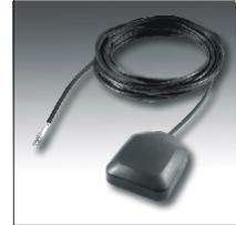
The antenna connects to the GPS connector of the MICOM transceiver through a 5-meter (15 feet) long coaxial cable, which is part of the antenna. This cable carries both DC power for the antenna, and the received GPS signals.
